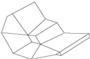
Fold down the winglets along fold lines 10. Now you are ready to fly! Hold the plane with your thumb against the nose and your index and middle finger behind cut line 5. Launch very gently from above your head.
