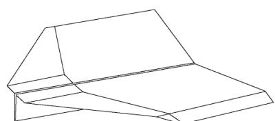
Fold the wings down along fold lines 7 and the winglets down along fold lines 8. Add wing dihedral by tilting the wings up slightly away from the fuselage. The wings will have a slight "V" shape when viewed from the front. You are ready to fly!
