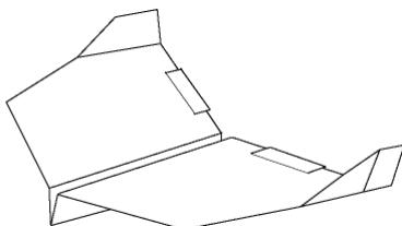
Flip the wings down along fold lines 6 and the winglets up along fold lines 7. Cut slits along the back wing edge for the elevator adjustment. Add wing dihedral by tilting the wings up slightly away from the fuselage. The wings will have a slight "V" shape when viewed from the front. You are ready to fly!
