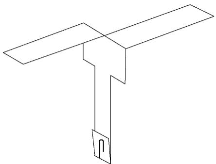
Fold rotors down along fold lines 6 in opposite directions. Attach a paper clip to the bottom tab to add weight. Drop from high over your head and watch the helicopter spin as it descends slowly.
