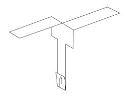
Fold rotors down along fold lines 6 in opposite directions. Attach a paper clip to the bottom tab to add weight. Drop from high over your head and watch the helicopter spin as it descends slowly.
