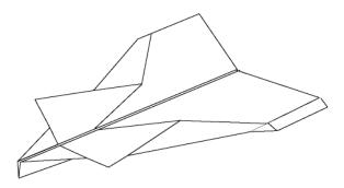
This unique plane has small wings at the front called "canards." This design is surprisingly stable and will float long and straight if folded carefully.
