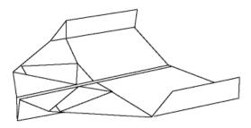
The Bulldog has a compact nose section that makes it very stable by keeping the center of gravity forward. It flies well indoors or in very light breezes outdoors.
